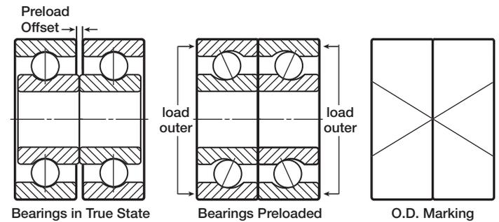
When face-to-face (DF) duplex pairs are mounted, the inner rings abut and the outer rings are drawn together, providing a higher radial and axial stiffness and accommodation of misalignment.
