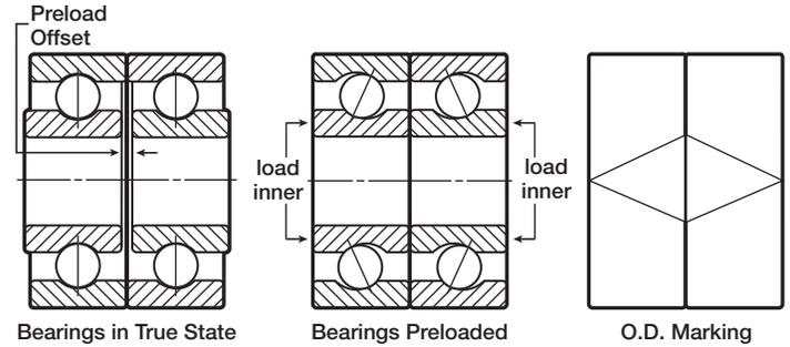
When a back-to-back (DB) duplex pair is mounted, the outer rings abut and the inner rings are drawn together, providing maximum stiffness.
