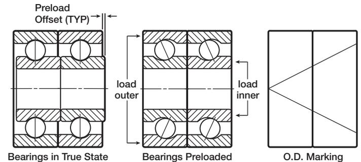
With tandem (DT) pairs, both inner and outer rings abut and are capable of sharing a thrust load, providing increased thrust capacity.
